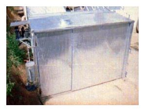
Picture 4. - Vacuum condensation dehydrator
